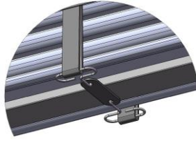
FUSIBLE LINK HOLDING BLADES OPEN
