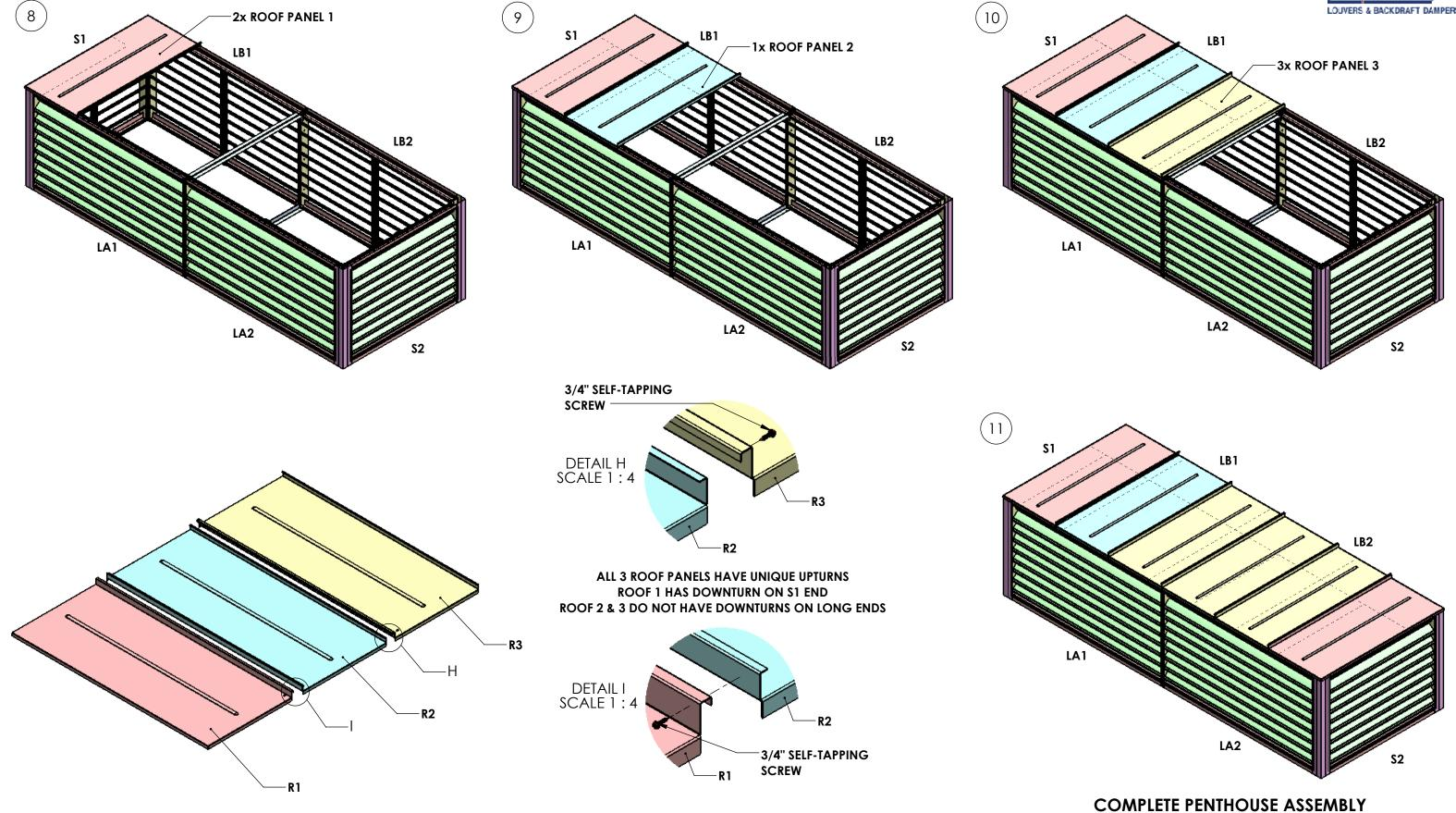
ASSEMBLE THE ROOF PANELS AS SHOWN
